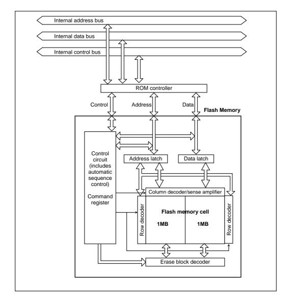
Fig. 3.1.2.1 Block Diagram of the Flash Memory Section
